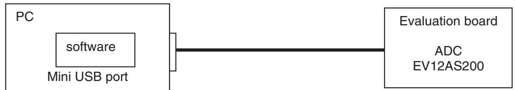
1. Use an mini USB port to send data to the ADC.
