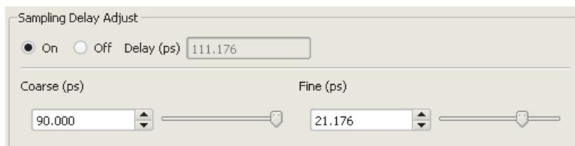
So the Sampling Delay adjusts with the 3WSI interface could vary from 0ps up to 120ps with a step of 0.12ps.
