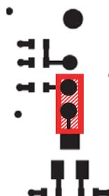
Jumper: Functionality activated -> Variation of voltage range with tuneable resistor between  $(2 \times V_{CC3}/3 - 0.5V = 1.7V)$  and  $(2 \times V_{CC3}/3 + 0.5V = 2.7V)$
