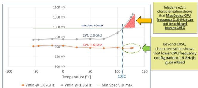
Fig. 5: CPU Frequency versus Supply voltage.
