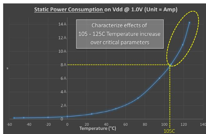
Fig. 4: Power Consumption versus Temperature.
