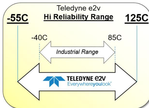
Fig. 1: Avionics, Space & Defense Temperature Requirements versus Industrial Grade.
