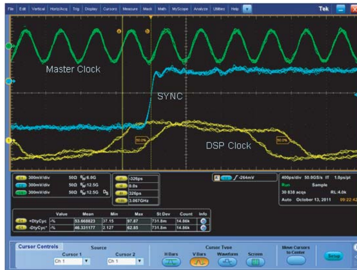
Figure 2-16. Example of Forbidden Zone at Fclk 2.5 GHz
