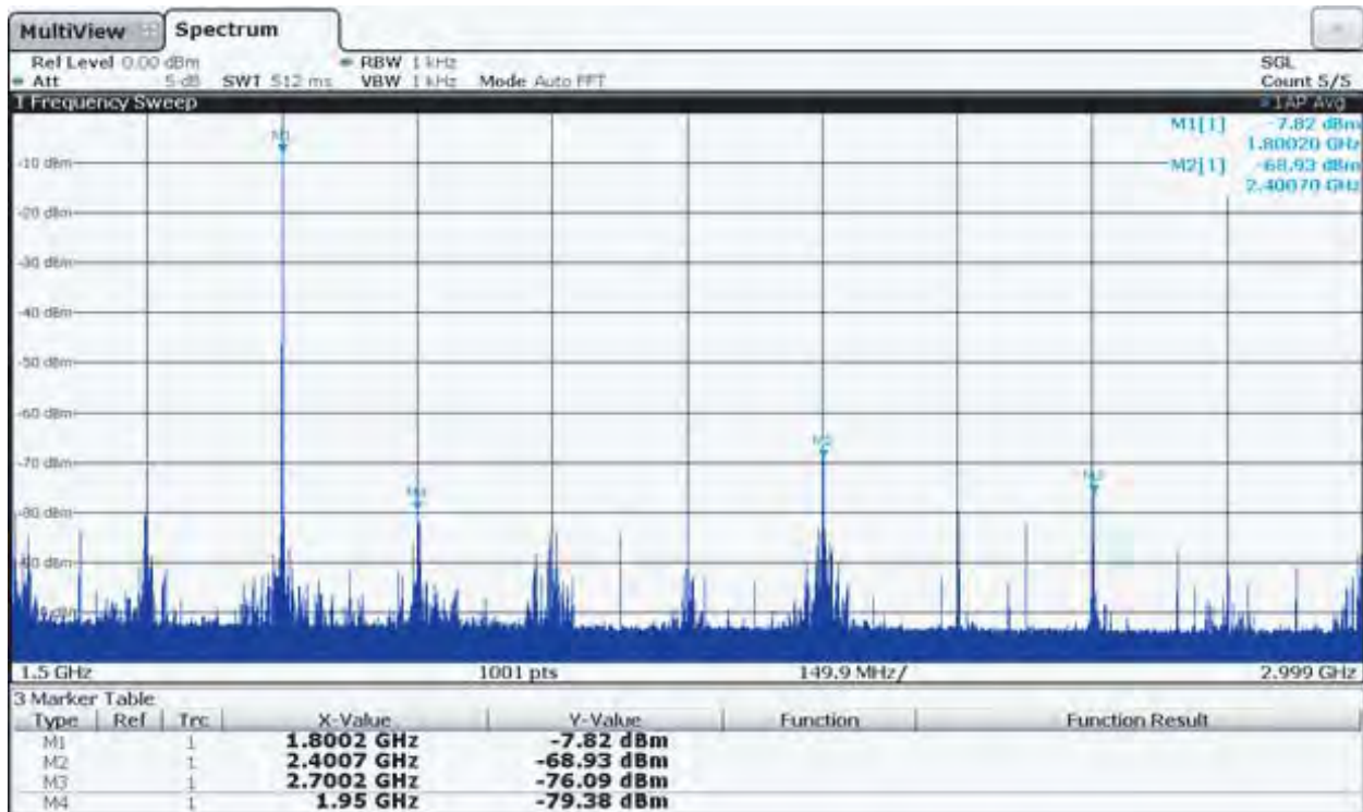
Figure 7-22. Typical SFDR spectrum in NRTZ mode. F_{out} = 1800\text{MHz} (2nd Nyquist), MUX4:1, F_s = 3\text{Gps} . SFDR = 61dBc
