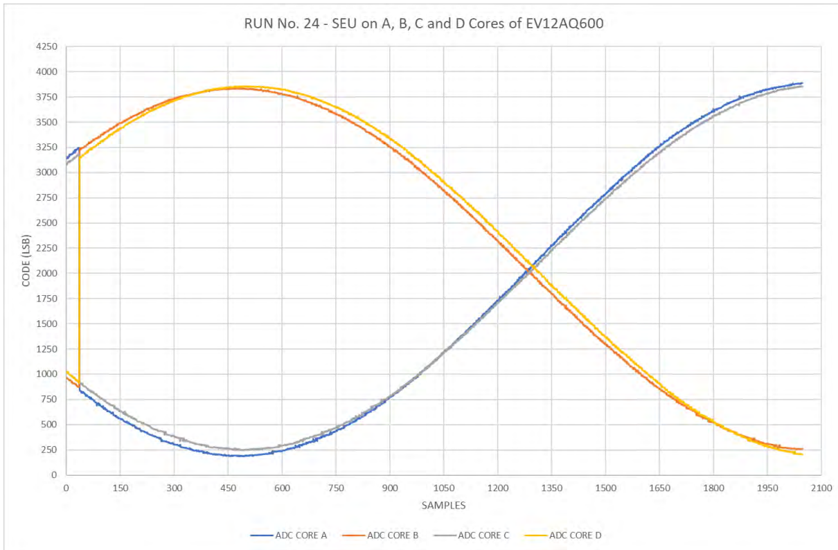
Figure 17: EV12AQ600 SEU case n°4 on A, B, C and D cores in MODE1 test configuration
