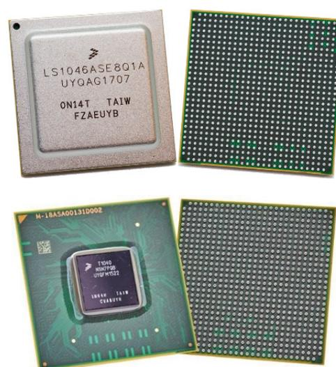
Figure 3: LS1046 lidded design [Top], T1040 lidless design [Bottom].
