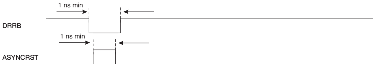
Figure 2-3. Reset Sequence (DRRB and ASYNCRST Not Simultaneous)
