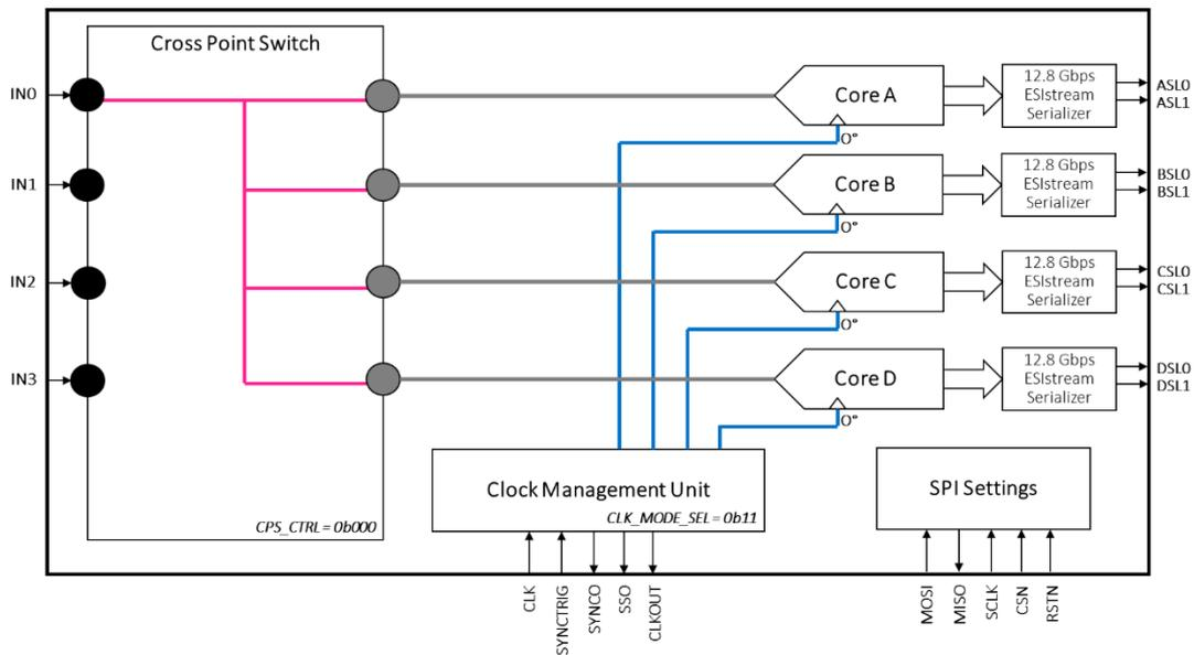
Figure 1 – CPS and clock mode configurations
