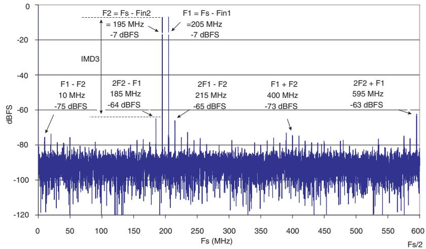
Note: The output data is not decimated. The spectrum is displayed from DC to 600 MHz.
