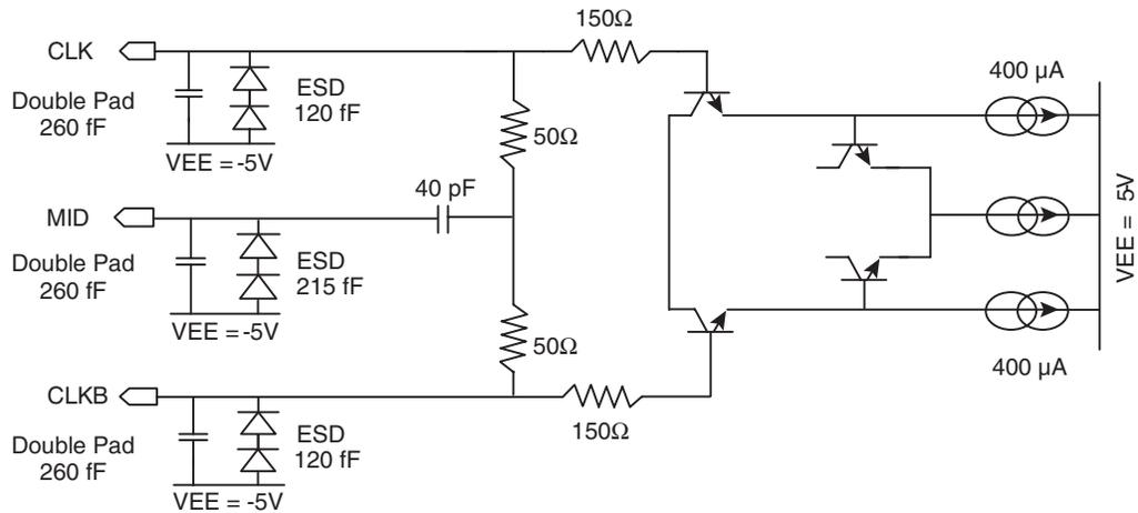
Note: 100Ω termination midpoint is on-chip and AC coupled to ground through a 40 pF capacitor.
