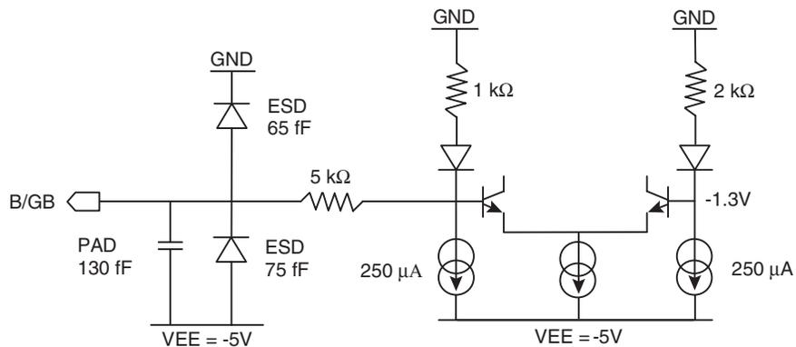
Figure 7-6. DRRB Equivalent Input Schematics and ESD Protections
