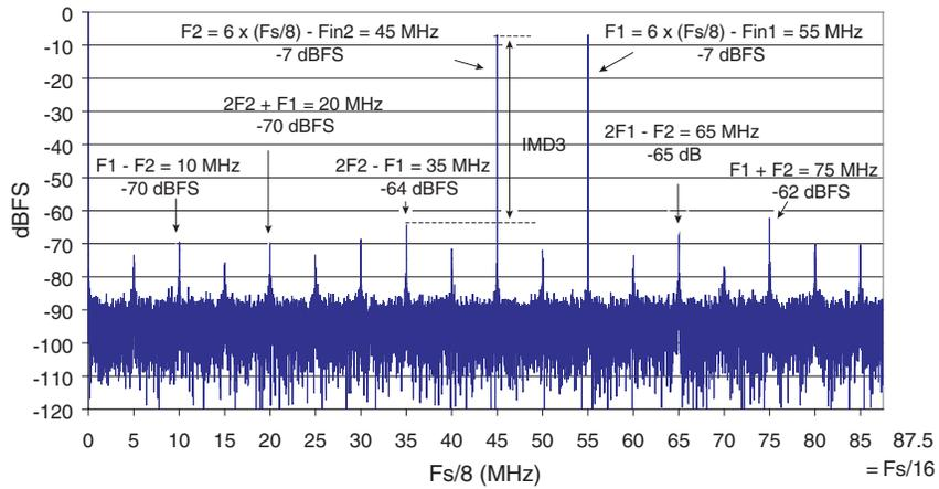
Note: The ADC input signal is sampled at 1.4 Gsps but the data acquisition is 8 times decimated. Thus, the spectrum is displayed from DC to  $F_s/2$  divided by the decimation factor  $[(F_s/2)/8 = 87.5$  MHz].
