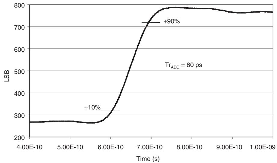
Note: Overshoot and ringback are not measurable (estimated by simulation at 4% and 2% respectively).
