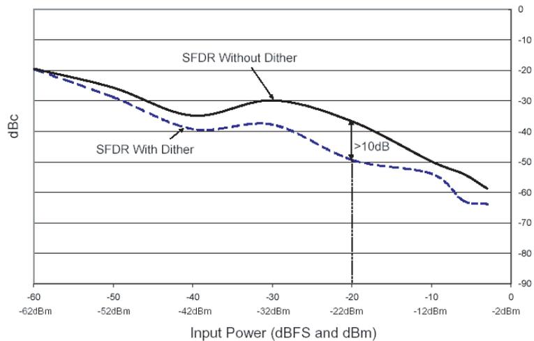
An increase in SFDR up to  $>10$  dB with an addition of  $-23$  dBrms DC to 5 MHz out-of-band dither is noted.
