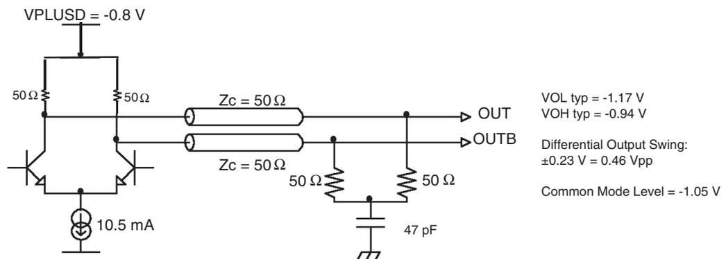
**Figure 9-8.** Underterminated Differential Outputs (Optional)
