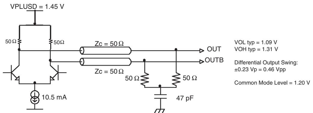
**Figure 9-10.** Underterminated Differential Outputs (Optional)
