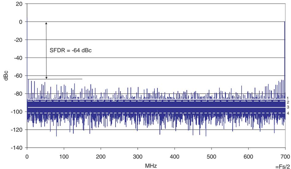
This is a 16384 points FFT. It is 16 times decimated since a DEMUX 1:8 is used to relax the acquisition system data rate, and data is captured on the rising edge of the data ready signal.
