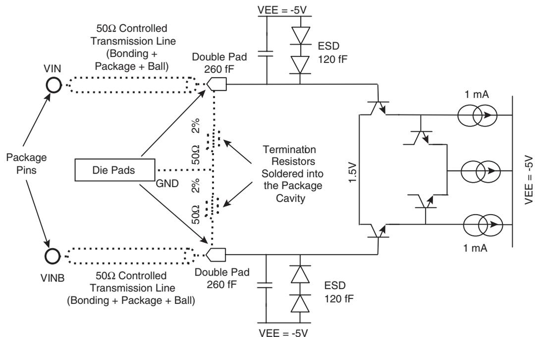
Note: 100Ω termination midpoint is located inside the package cavity and is DC coupled to ground.
