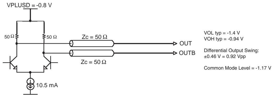
9.6.2 LVDS Differential Output Loading Configurations
