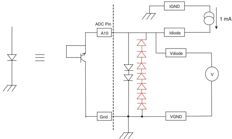
**Figure 9-13.** Diode Pin Implementation for Decimation Activation
