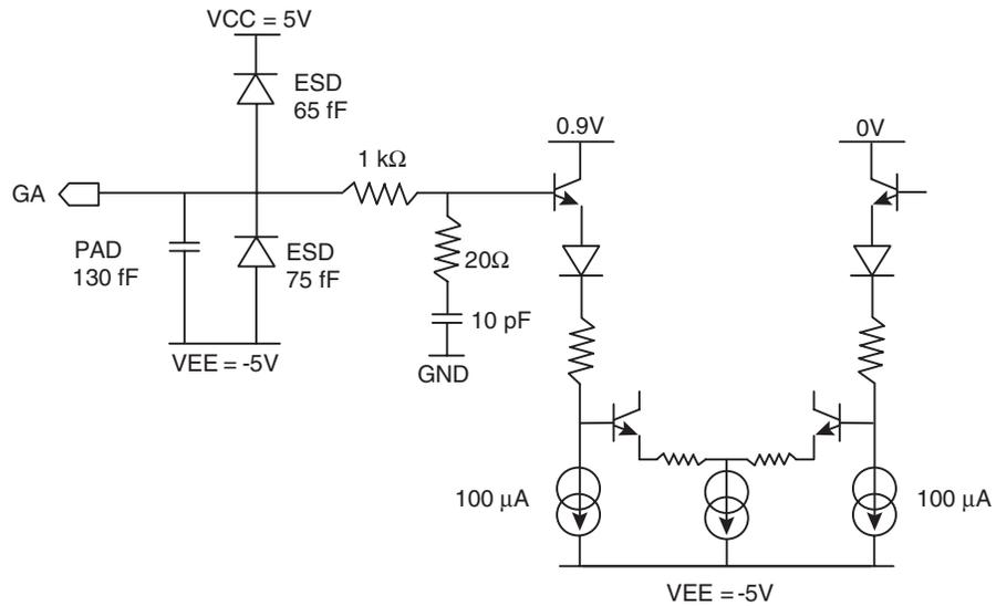
Figure 7-5. B/GB and PGEB Equivalent Input Schematics and ESD Protections
