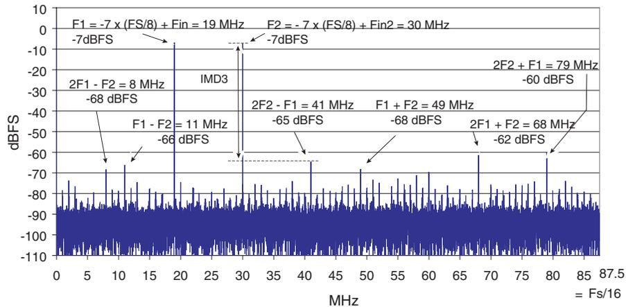
Note: The ADC input signal is sampled at 1.4 Gsps but data acquisition is 8 times decimated. Thus, the spectrum is displayed from DC to  $F_s/2$  divided by the decimation factor  $[(F_s/2)/8 = 87.5$  MHz]. The dual tone  $IMD3$  at 1.4 Gsps is around  $-65$  dBFS for  $F_{in} = 1$  GHz  $\pm 250$  MHz ( $F_{in}$  range is from 750 MHz to 1250 MHz).
