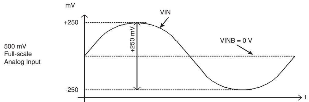
The analog full-scale input range is 0.5V peak-to-peak ( $V_{pp}$ ), or  $-2$  dBm into the  $50\Omega$  ( $100\Omega$  differential) termination resistor.
