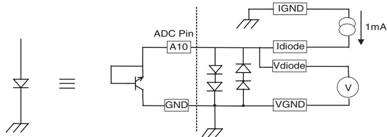
9.7.7 Junction Temperature Diode Transfer Function
