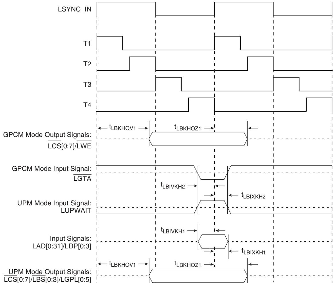
**Figure 10-7.** Local Bus Signals, GPCM/UPM Signals for LCCR[CLKDIV] = 8 or 16 (PLL Bypass Mode)
