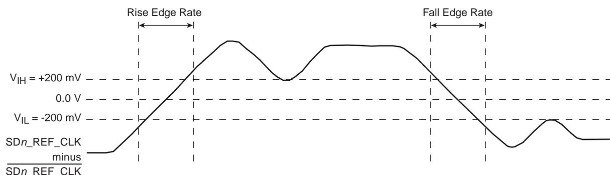
**Figure 15-11.** Single-Ended Measurement Points for Rise and Fall Time Matching
