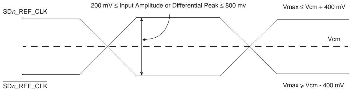
**Figure 15-5.** Single-Ended Reference Clock Input DC Requirements
