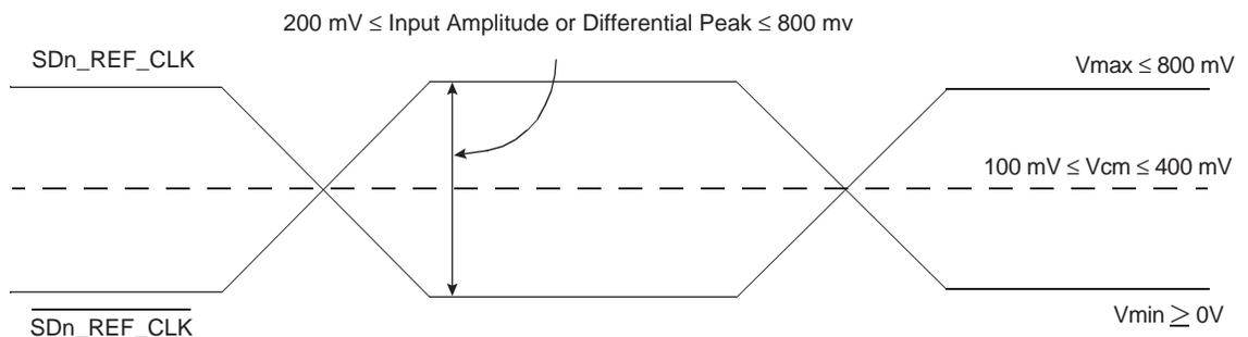
**Figure 15-4.** Differential Reference Clock Input DC Requirements (External AC-Coupled)
