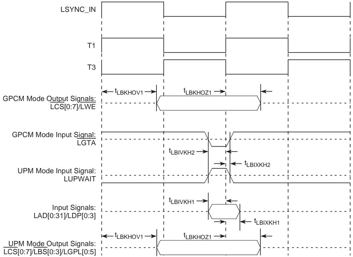
Figure 10-5. Local Bus Signals, GPCM/UPM Signals for LCCR[CLKDIV] = 4 (PLL Bypass Mode)
