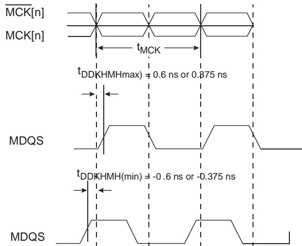
Figure 6-3 shows the DDR2 and DDR3 SDRAM Interface output timing diagram.
