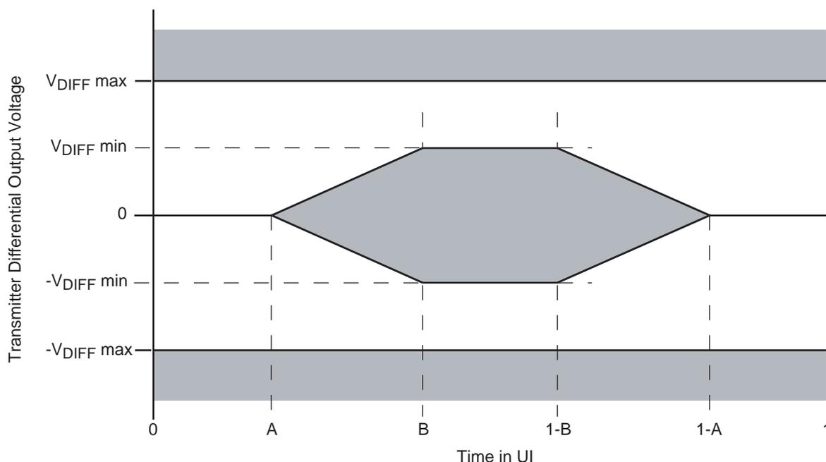
**Table 17-8.** Transmitter Differential Output Eye Diagram Parameters
