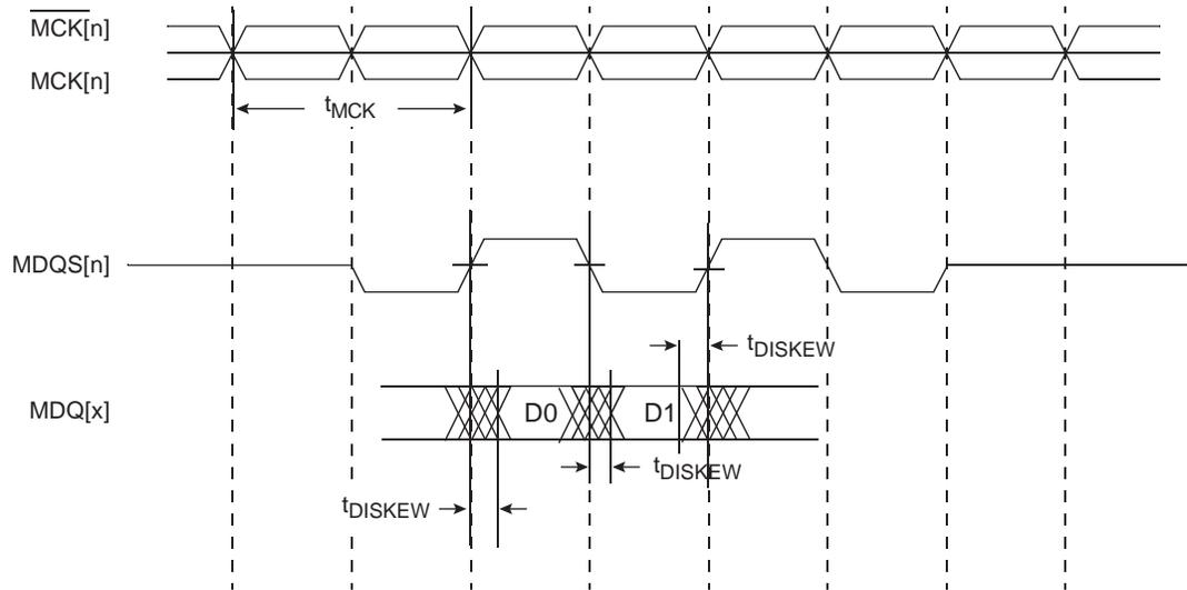
**6.2.2 DDR2 and DDR3 SDRAM Interface Output AC Timing Specifications**
