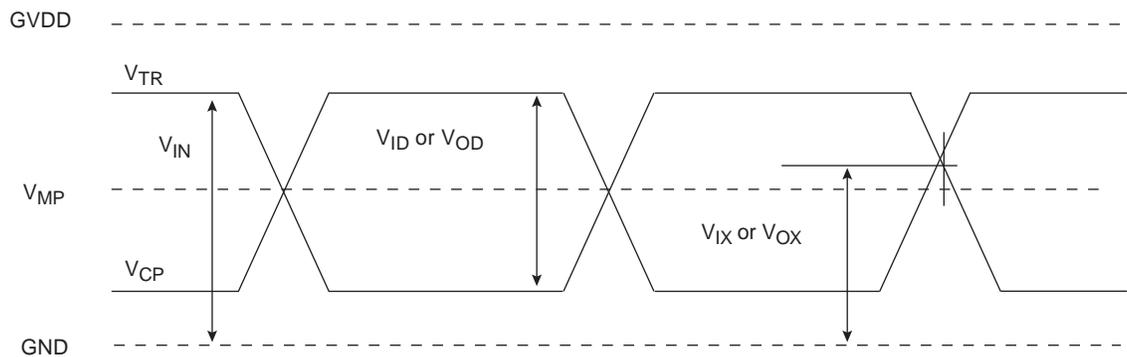
Note:  $V_{ID}$  specifies the input differential voltage  $|V_{TR} - V_{CP}|$  required for switching, where  $V_{TR}$  is the true input signal (such as  $MCK$  or  $MDQS$ ) and  $V_{CP}$  is the complementary input signal (such as  $\overline{MCK}$  or  $\overline{MDQS}$ ).
