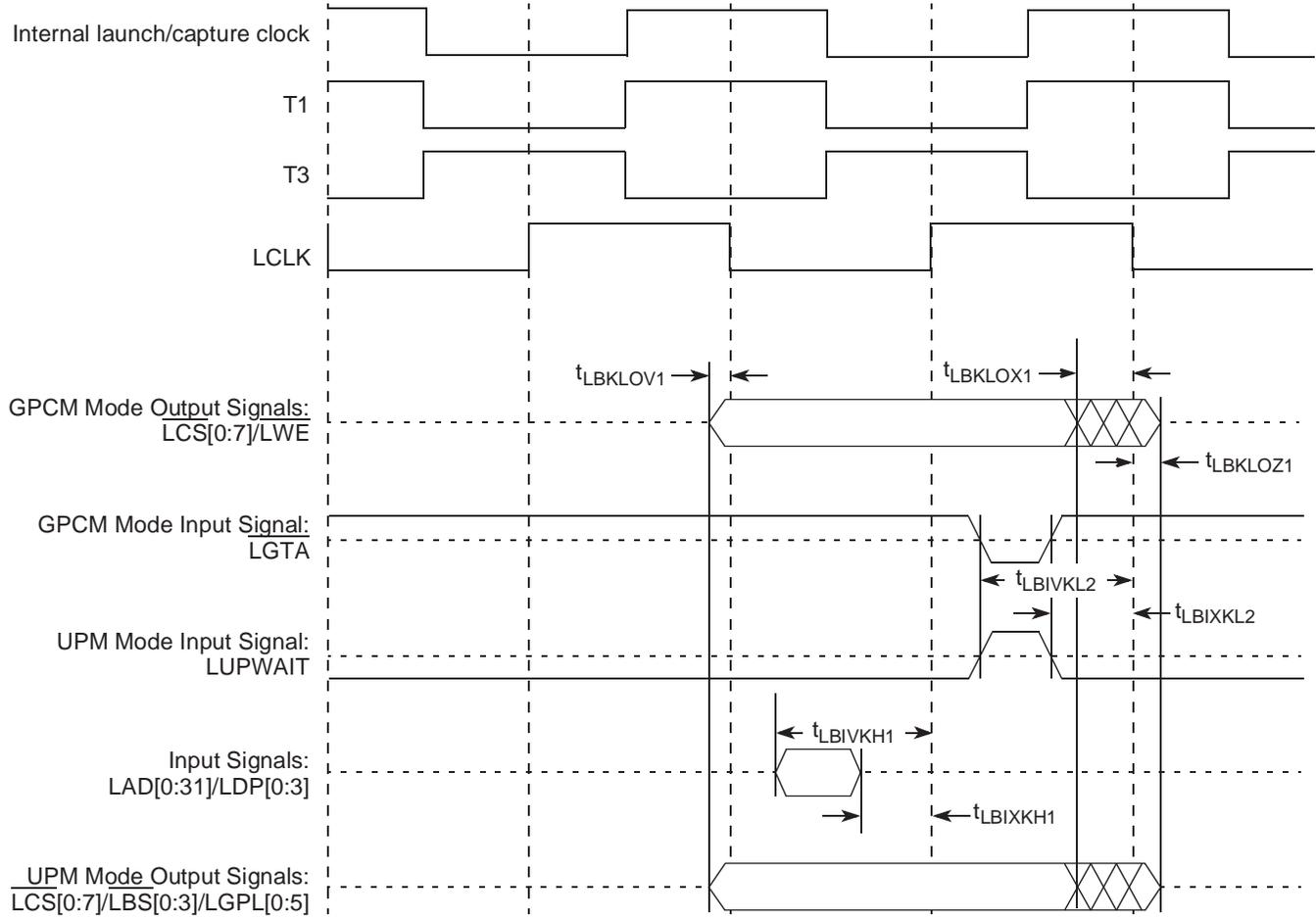
Figure 10-6. Local Bus Signals, GPCM/UPM Signals for LCCR[CLKDIV] = 8 or 16 (PLL Enabled)
