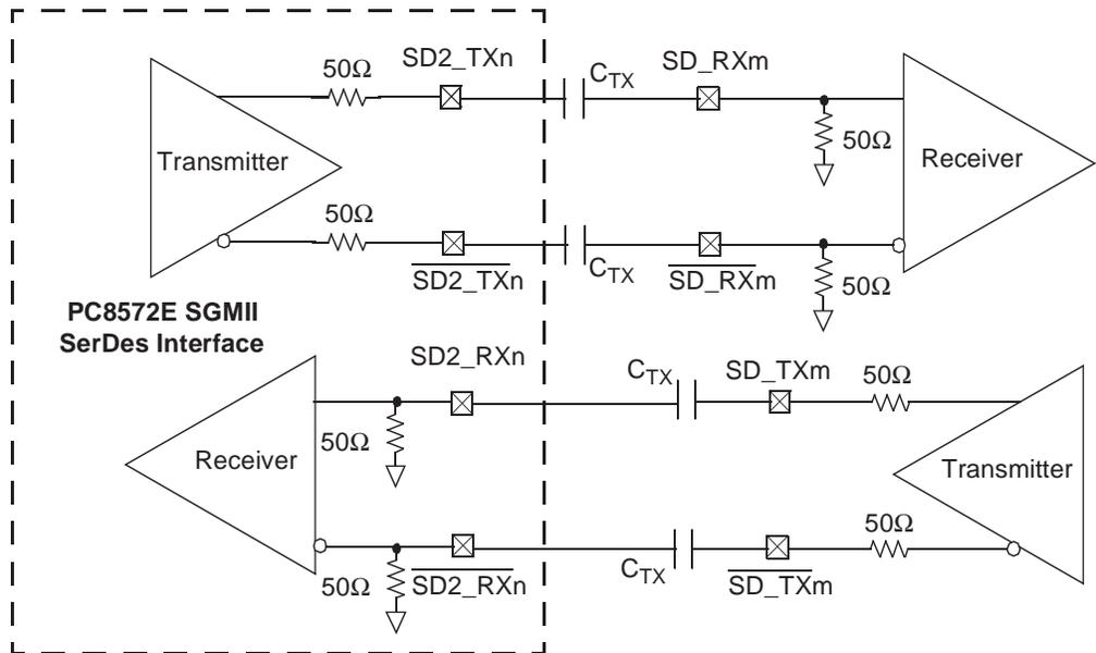
Figure 8-17. SGMII Transmitter DC Measurement Circuit
