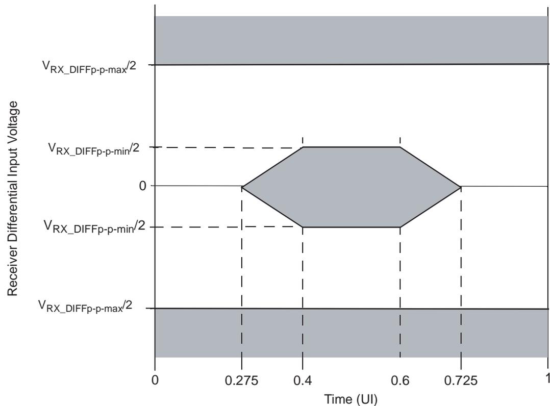
Figure 8-19. SGMII AC Test/Measurement Load
