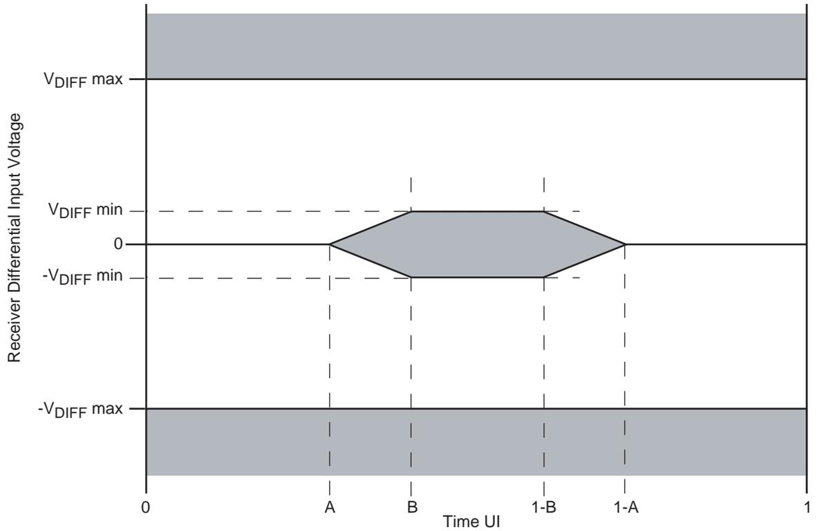
Table 17-12. Receiver Input Compliance Mask Parameters Exclusive of Sinusoidal Jitter
