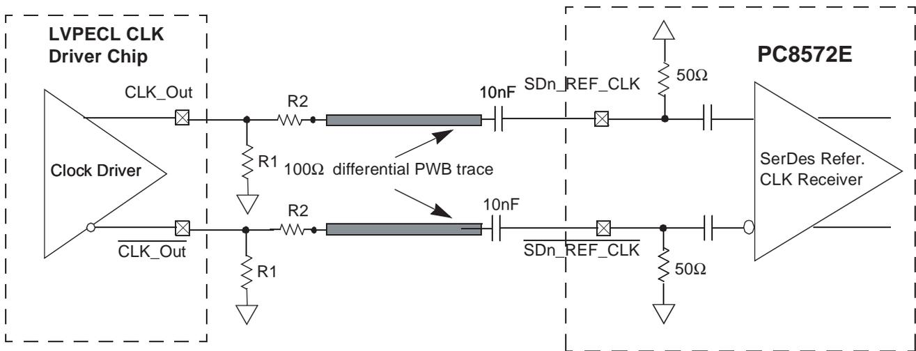
Figure 15-9 shows the SerDes reference clock connection reference circuits for a single-ended clock driver. It assumes the DC levels of the clock driver are compatible with PC8572E SerDes reference clock input's DC requirement.
