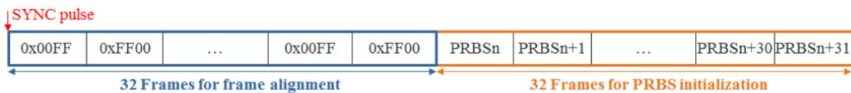
Figure 7 ESistream Link synchronization frames.
