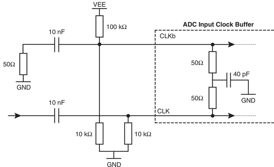
In the case of an application requiring a fixed clock frequency, it is recommended to filter the clock signal for improved jitter performance. The benefits of filtering the clock signal can be quantified to a 1 or 2 dB improvement in the SNR figure and thus in an increase of about 0.1 to 0.2 bit in the ENOB figure.
