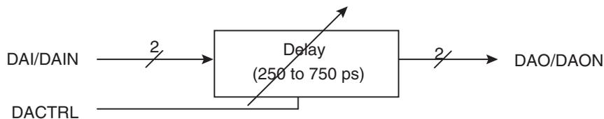
The input buffer for DAI/DAIN is described in [Figure 4-3 on page 10](#). As it is on-chip already +2 x 50Ω terminated the 100Ω LVDS external termination is not required.
