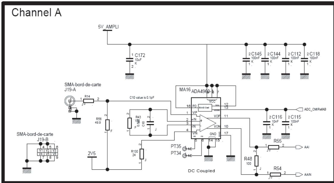
The ADA4960 is used in DC configuration with output common mode driven by ADC QUAD 10-bit. The input is biased at 2.5V since this is a requirement for best performance from the amplifier, this should be taken into account when using this input.
