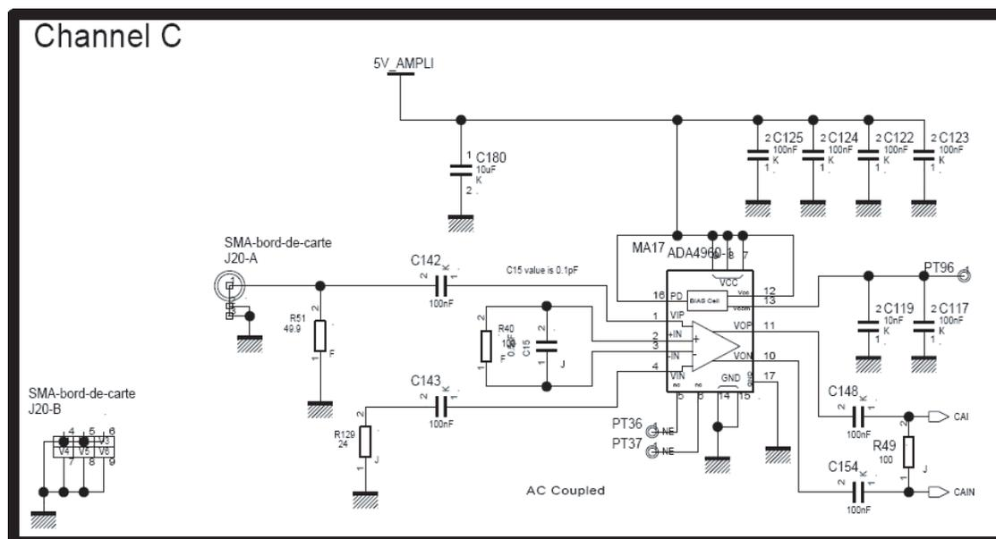
The ADA4960-1 is used in AC configuration with output common mode driven by Quad 10-bit ADC.
