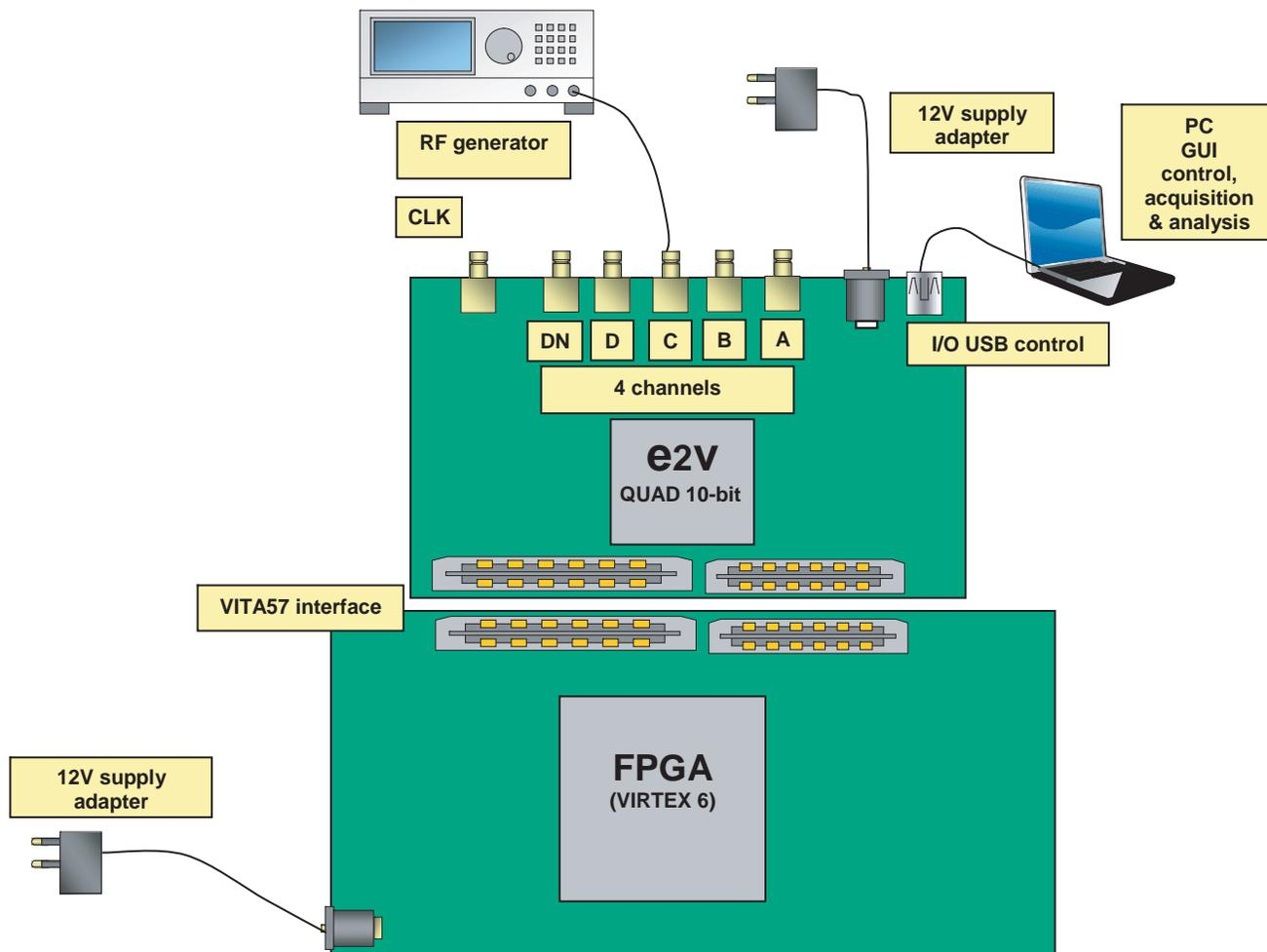
The complete system is built with the e2v demo kit and an FPGA development kit. e2v Demo kit contains the following items :
