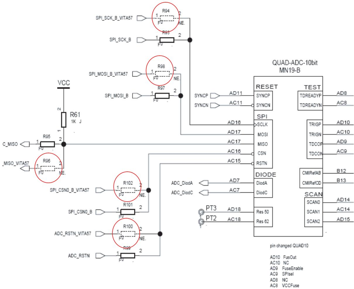
Figure 6-5. Implantation of R93, R94, R95, R96, R97, R98, R99, R100, R101 and R102 resistors
