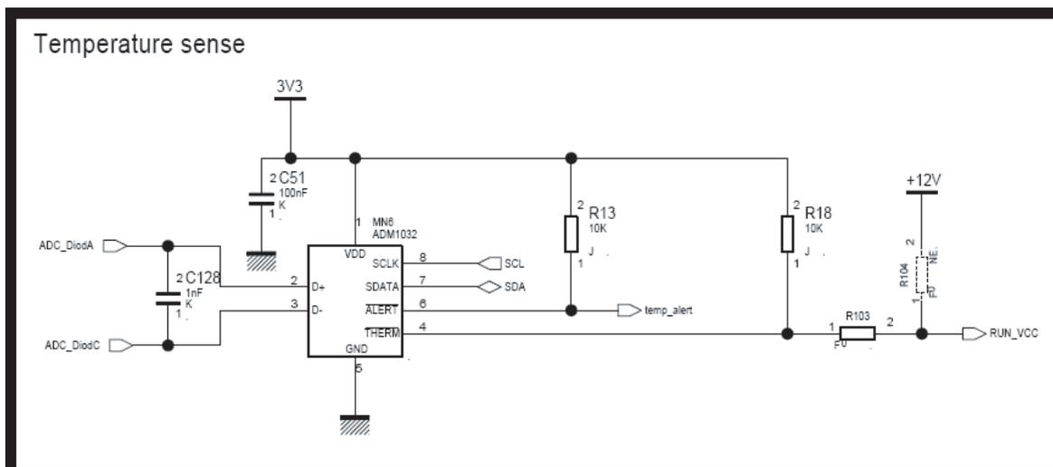
ADC junction temperature can be displayed on the PC via the GUI with a resolution of  $\pm 2^{\circ}\text{C}$ . Please see Section 4.5.5 Power.
