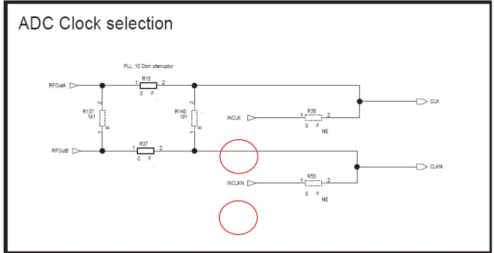
Figure 6-3. Implantation of R15, R37, R36 and R50 Resistors
