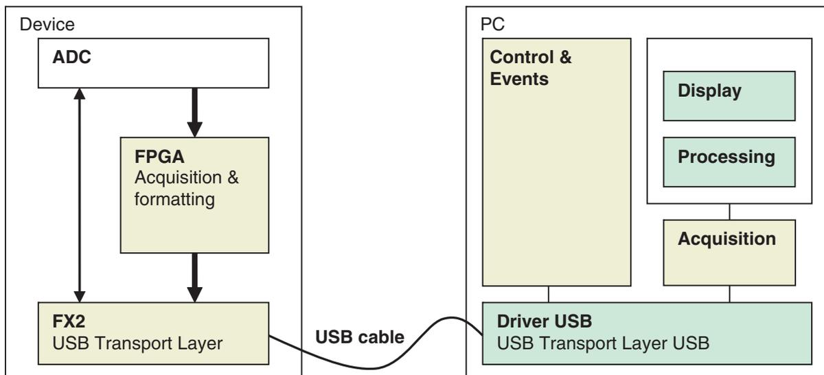
Acquisition and formatting of ADC digital output data are done within the FPGA Eval Kit. Data is then transmitted again to the ADC Demo Kit.
