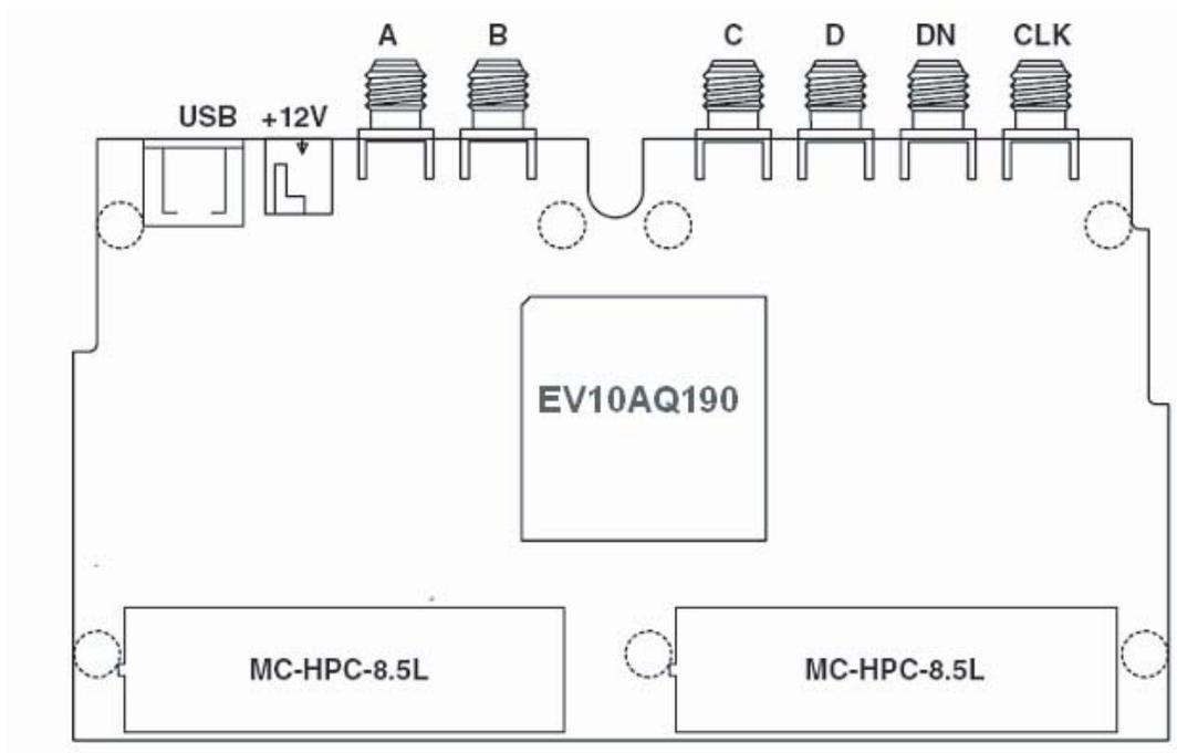
Figure 1-4. EV10AQ190x-DK Demo Kit Functional Architecture
