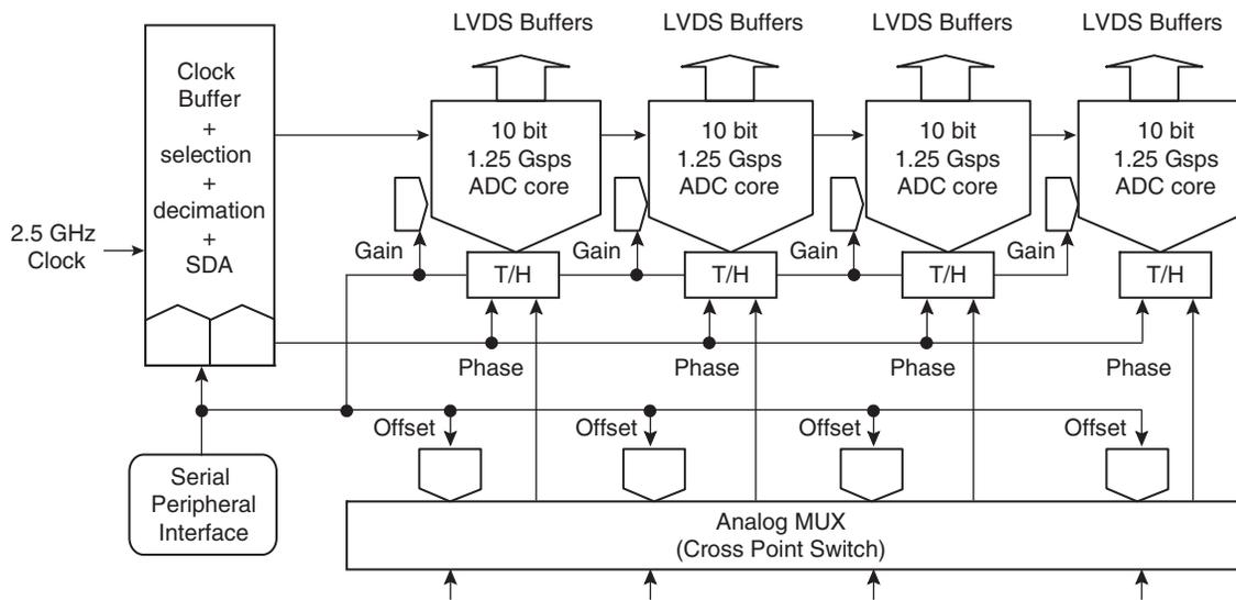
The EV10AQ190x Quad 10-bit ADC integrates four 10-bit ADC cores which can operate independently (four-channel mode) or group by two cores (two-channel mode with the ADCs interleaved two by two) or one-channel mode where all four ADCs are all interleaved.
