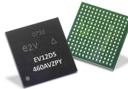
This DAC provides an analog bandwidth beyond 7GHz and contains a flexible input multiplexer guaranteeing sampling rates at 6 GSps with the ability to operate at 7 GSps.
