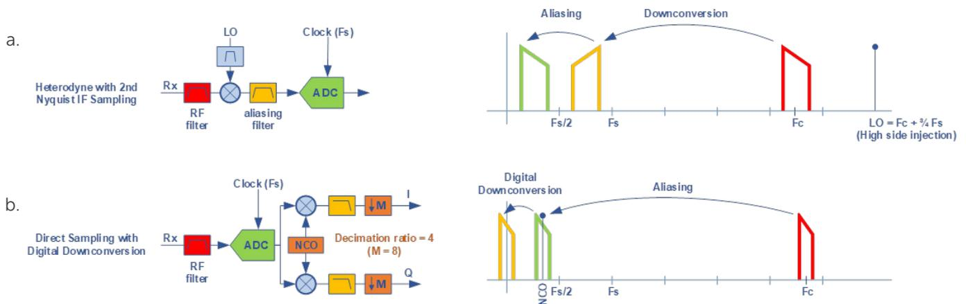
Figure 1 - Simplified Rx signal chains in a) traditional single stage heterodyne radio with mixer down conversion and b) a direct conversion system exploiting sampled signal aliasing within the ADC.
