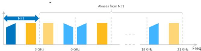
Figure 4 - Synthetic RF signal generated in  $NZ_1$  and aliased into higher order Nyquist zones ( $f_s = 6$  GHz).
