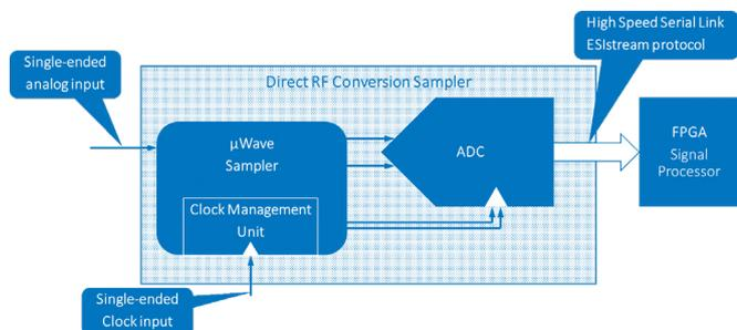
Figure 5 - Prototype direct conversion RF sampler.
