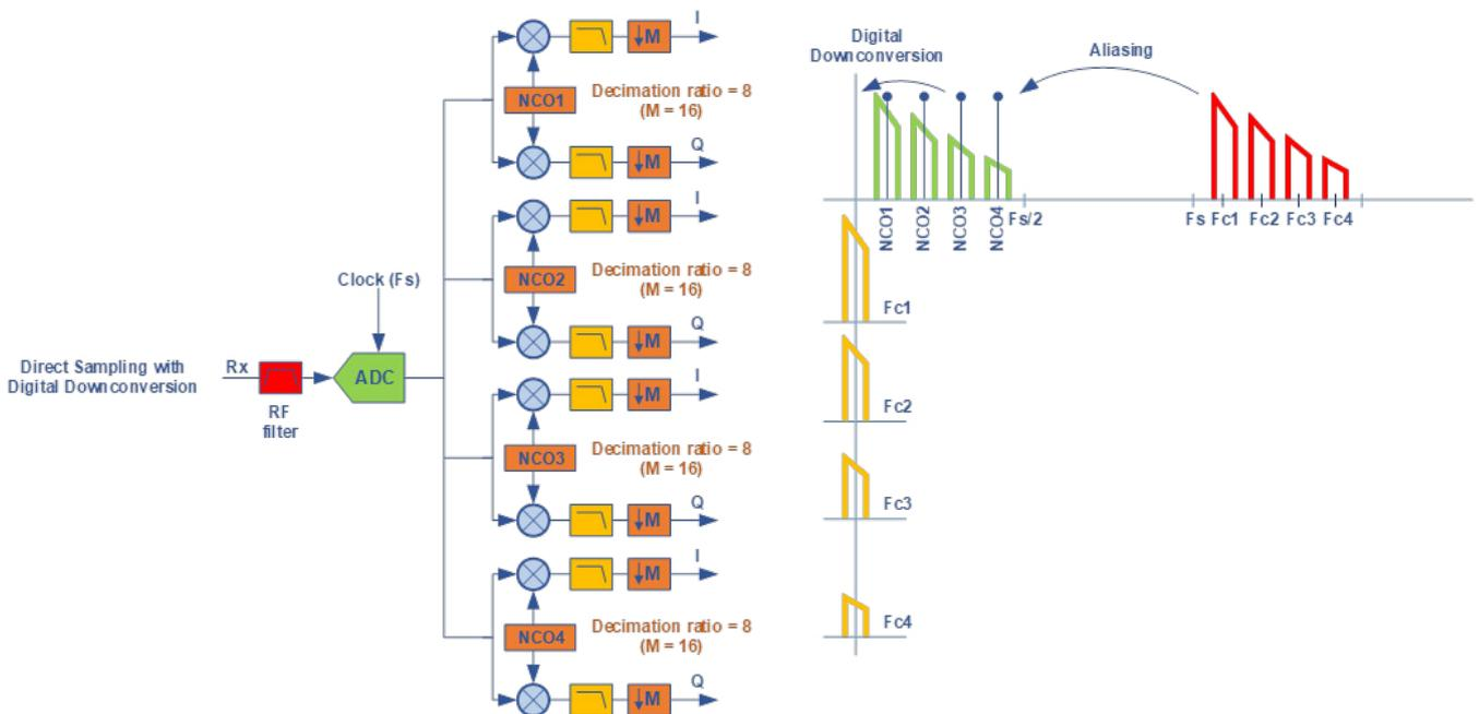
Figure 2 - In an enhanced SDR, numerical controlled oscillators can tune to any number of separate channels as shown.
