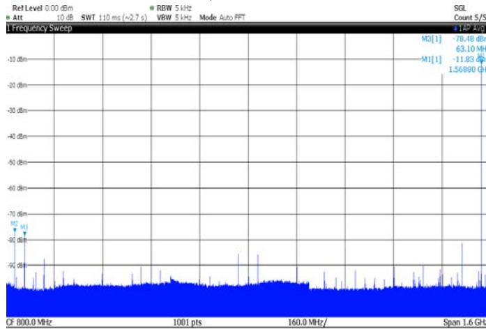
Figure 7-33. Typical SFDR spectrum in NRTZ mode. Fout = 1568 MHz (1 st Nyquist), MUX2:1, Fs = 3.2 GSps. SFDR = 65 dBc
